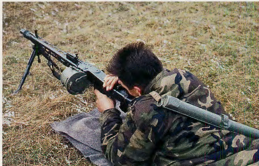
MG42 remains to this day an excellent machine gun. Note 50-round "basket" belt carrier and spare barrel carrier.
